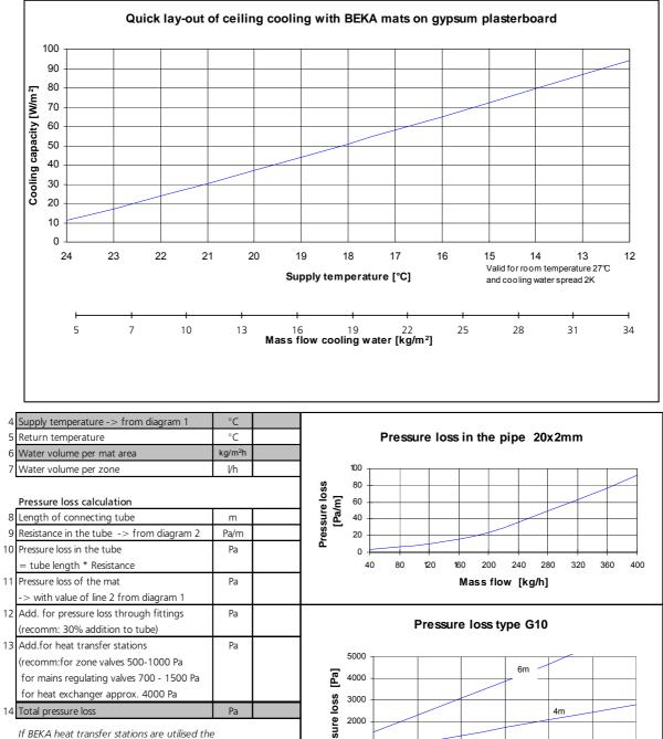
determination of pressure loss can be omitted. In this case only the quantity of cooling circuits and the total cooling capacity is required for the selection !
