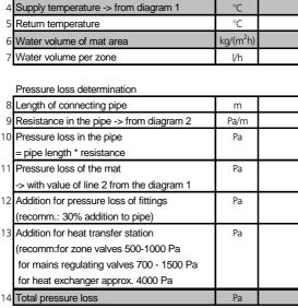
If BEKA heat transfer stations are utilised, the pressure determinaton can be omitted. Only the quantity of cooling circuits and the total cooling capacity is required for the selection.
